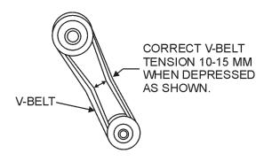
Figure 9. V-Belt Tension
